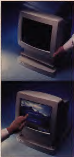
Users simply set their monitors on TouchMate to turn them into touch screens.
